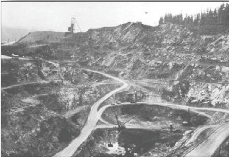
Brynnor Mine Open Pit with headframe in 1965. Jointing in sheeted dikes dips to left in headwall (Eastwood, 1968; Plate VII, p. 67)
